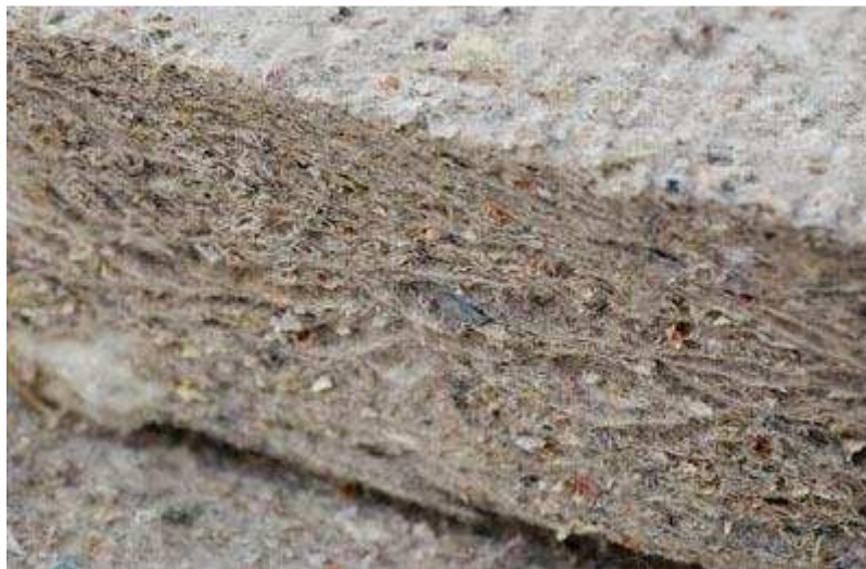
Figure 6: Illustration of cellulose insulation panels
