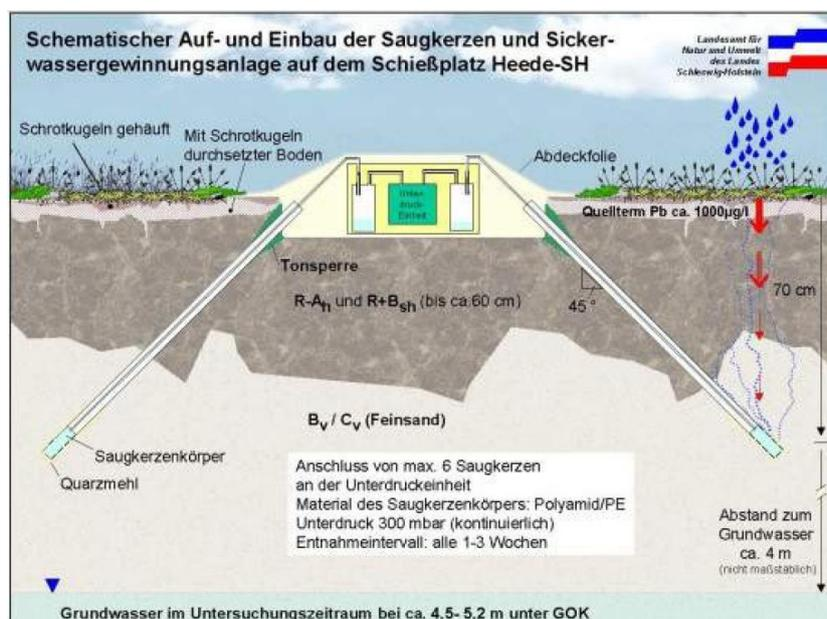
**Figure 1-12: Example for measurement of seepage water in a shooting range (Schleswig-Holstein LANU, 2005)**
