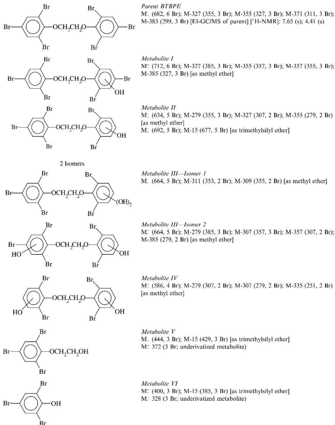
**Figure 19 Metabolites observed in the study of Hakk *et al.* (2004). Figure taken from Hakk *et al.* (2004).**
