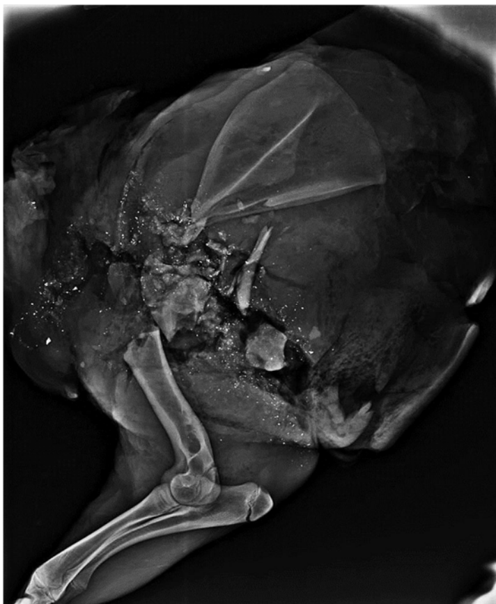
Figure B.9-9: X-Ray image of a wild boar skull hit by a bonded bullet (Swedish NFA, 2014a)
