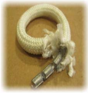
Lead rosary for internal ballasting of rope.
