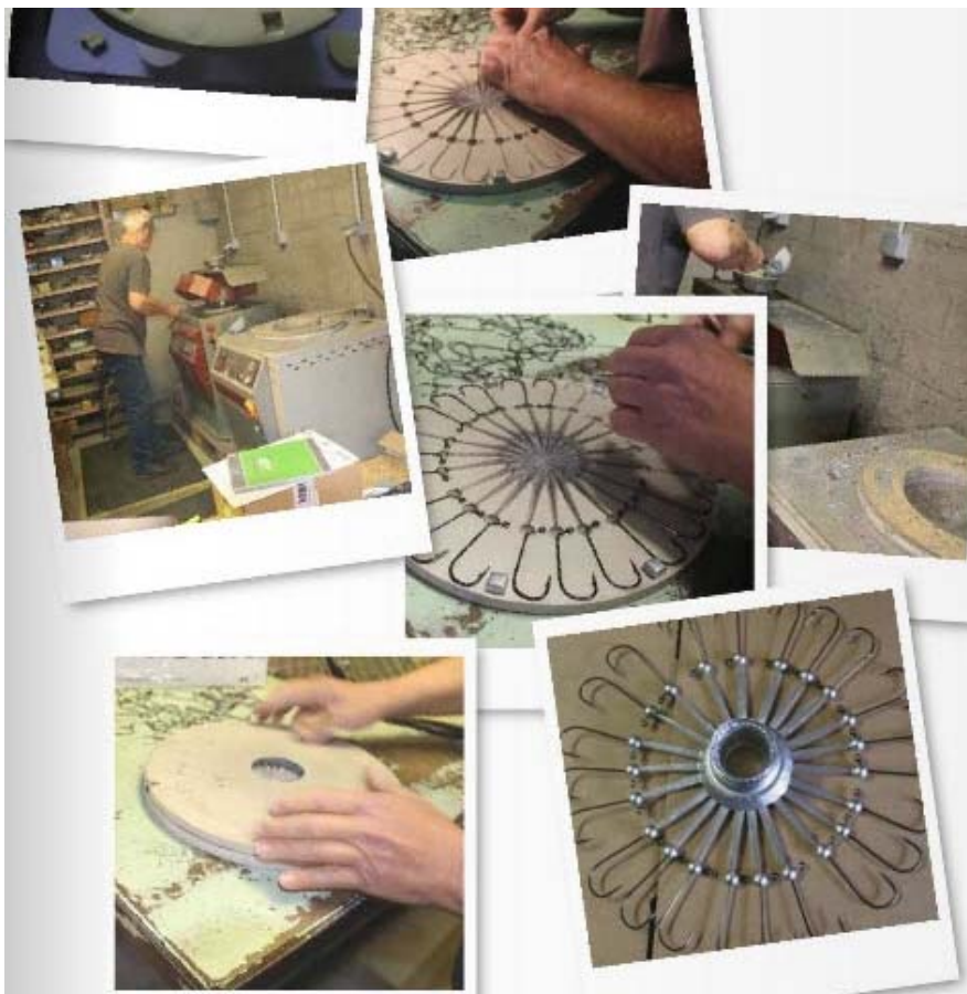
Figure A.2-6: Step by step instructions to home-cast fishing lure
