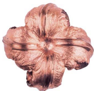
Figure D.1-12: Barnes TSX, TTSX, MRX expanded. Picture Federal Cartridge Co.
