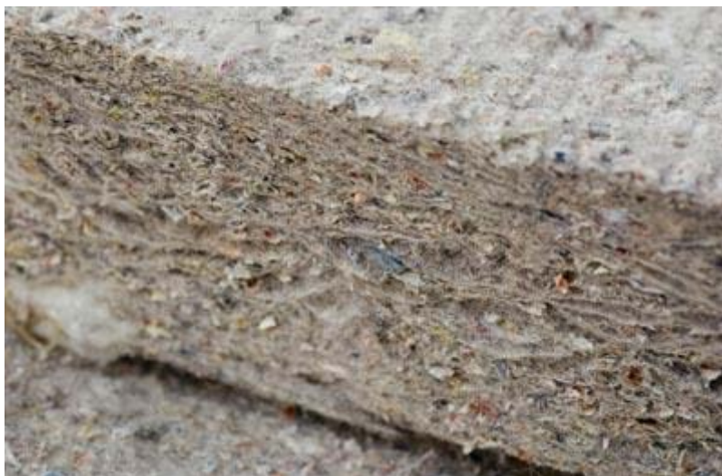
Figure 6: Illustration of cellulose insulation panels
