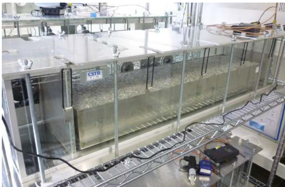
Figure 8: Cellulose insulation test specimen in a test chamber (CSTB 2013)
