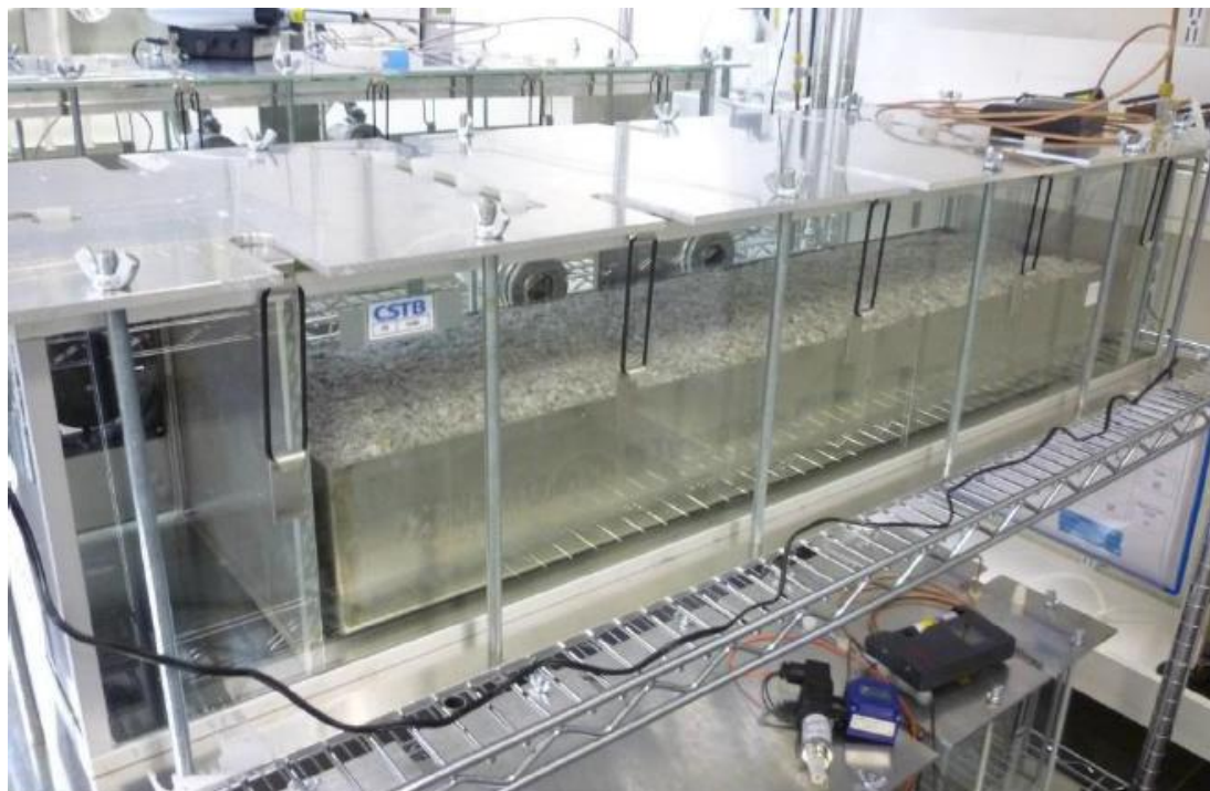
Figure 8: Cellulose insulation test specimen in a test chamber (CSTB 2013)
