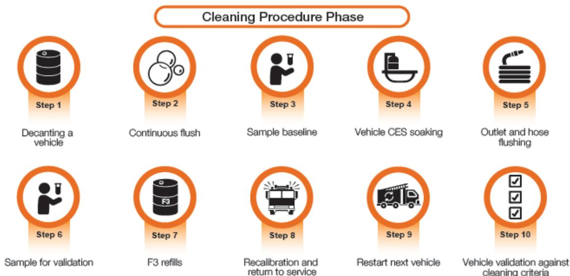
**Figure 7. Cleaning procedure phases in accordance to the Queensland DoD (DoD-AUS, 2020c)**
