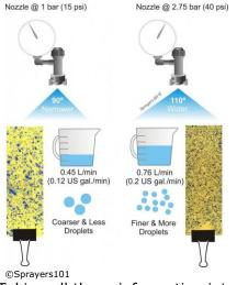
Using a flat fan nozzle as an example, **a lower pressure increases the median droplet diameter**, reduces the droplet count, reduces the nozzle flow rate and typically reduces the spray angle. Alternately, a higher pressure decreases the median droplet diameter, increases the droplet count, increases the nozzle flow rate and typically increases the spray angle.
