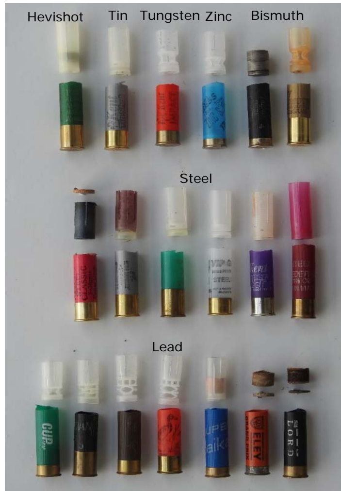
Figure E.8. Wad construction in a selection of shotgun cartridges. All calibre 12. Bottom: Lead; Middle: Steel; Top (from left): Hevishot, Tin, Tungsten, Zinc and two Bismuth. See text for details.
