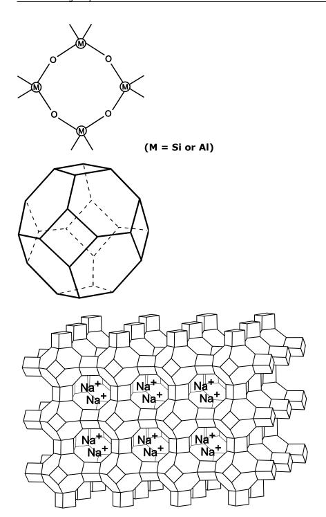
Upper: four membered ring structural unit of the zeolite A lattice; middle: Truncated octahedron of four- and six membered rings in the zeolite A lattice; lower: Zeolite A Lattice, in Sodium Form
